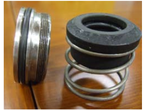
Corrosion of non-genuine shaft seals. A cheap purchase, but expensive to replace.
