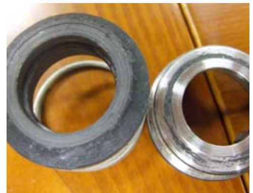
Low-quality non-approved seals present risk and lead to pump failure.
