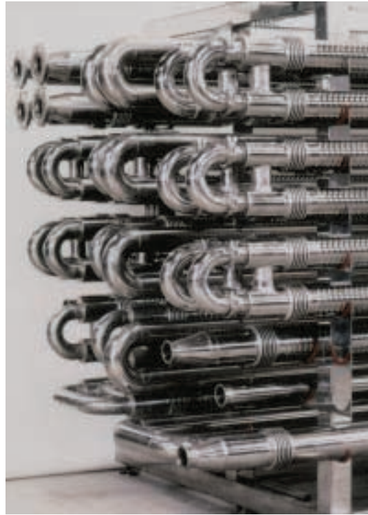
The ViscoLine tubular heat exchanger connected in series and grouped on a common frame
